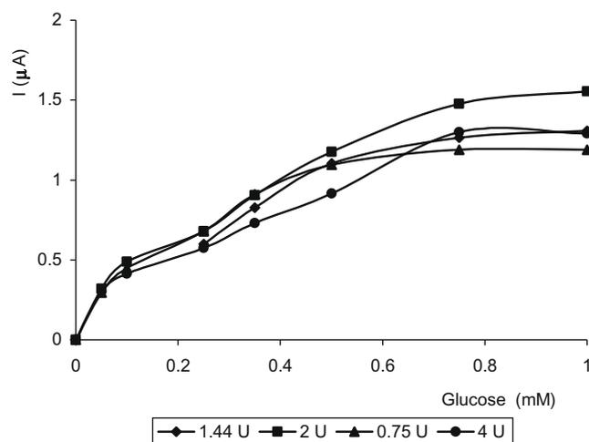
Fig. 2. Effect of enzyme loading on the biosensor response (potassium phosphate buffer: 50 mM, pH 6.5, -0.7 V).
