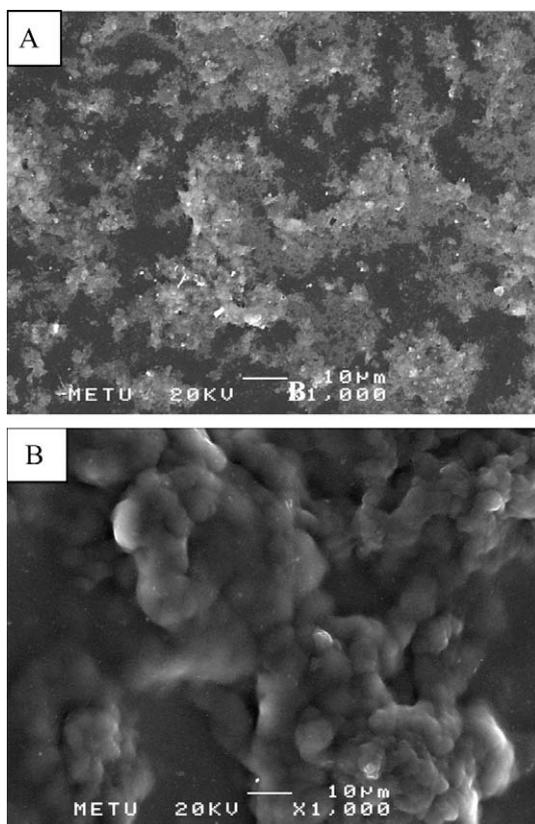
Fig. 1. SEM images of AuNPs-polyaniline/AgCl (A) and AuNPs-polyaniline/AgCl/gelatin (B) matrices.
