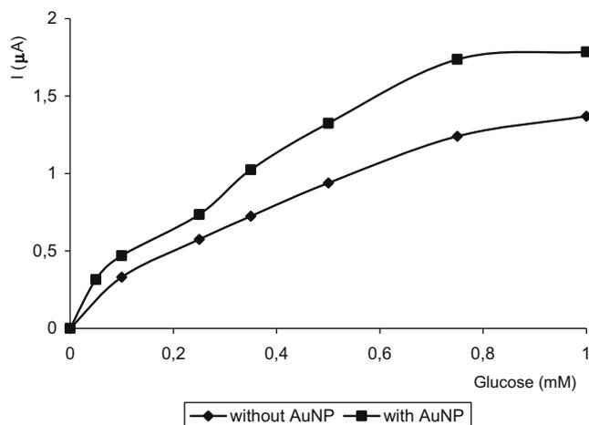
Fig. 3. Effect of AuNPs on the biosensor response (potassium phosphate buffer: 50 mM, pH 6.5,  $-0.7$  V).
