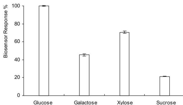
Fig. 4. Carbohydrate analysis using PyOx biosensor (potassium phosphate buffer: 50 mM, pH 6.5,  $-0.7$  V, sugar substrate: 0.25 mM).
